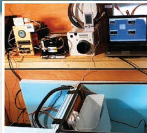
Temperature sensors fed into data-logging software on a laptop to chart cooling efficiency.
